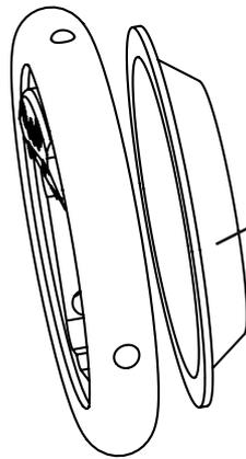
Fingerguard is securely fixed to the handwheel and not worn
